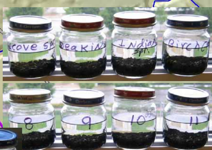
Figure 20. Photos of dye eluted from charcoal packets at springs from Meyer Well #48 Trace #2. Note the visual confirmation of dye in samples MG-1 through MG-5 but lab analysis also confirms dye in samples MG-14, MG-13, MG-12, MG-6 and MG-7 which are below the visual detection limit. Dye concentration needs to reach about 75 to 100 ppb before it can be detected with the unaided eye under natural light conditions. The left (MG-13) and right side (MG-7) of the purple line show the approximate spatial distribution of dye at the springs.
